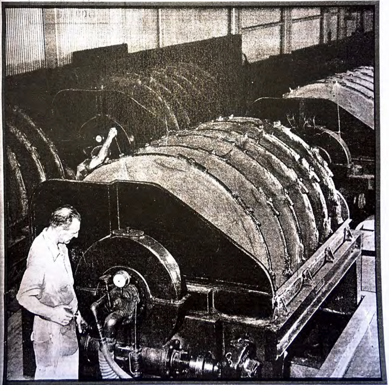
Continuous filtering on multiple-disc machines at Broken Hill, Australia
