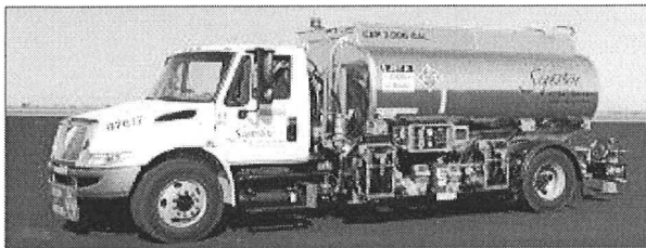
3000 Gallon Jet Refueler on International Chassis
