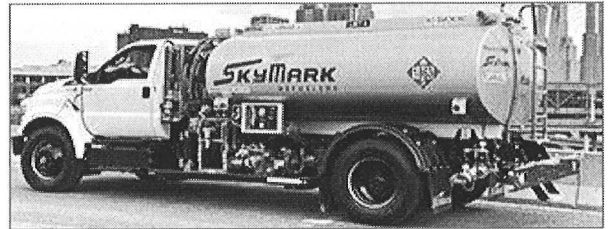
3000 Gallon Jet Refueler on Ford F-750 Chassis
