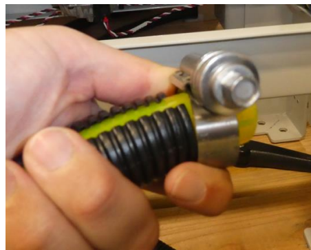
Figure 6: Hose with loom cut back (4X)
