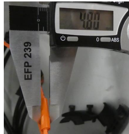
Figure 17: Item 11 Wrap around cable (4X)
