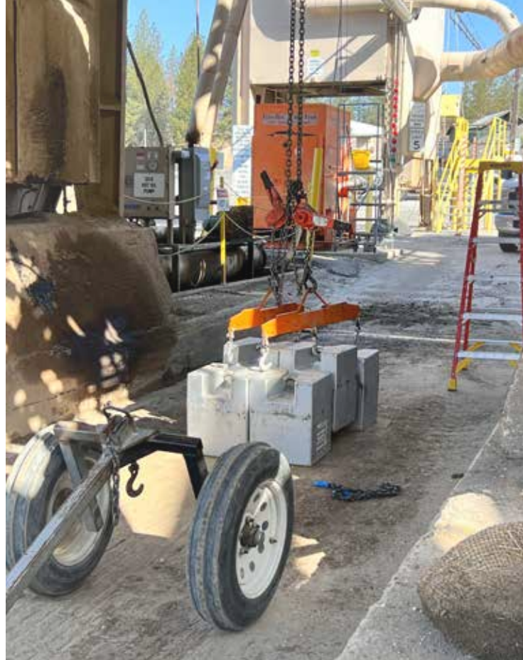
Testing the accuracy of hopper scales for asphalt mixing plant.
