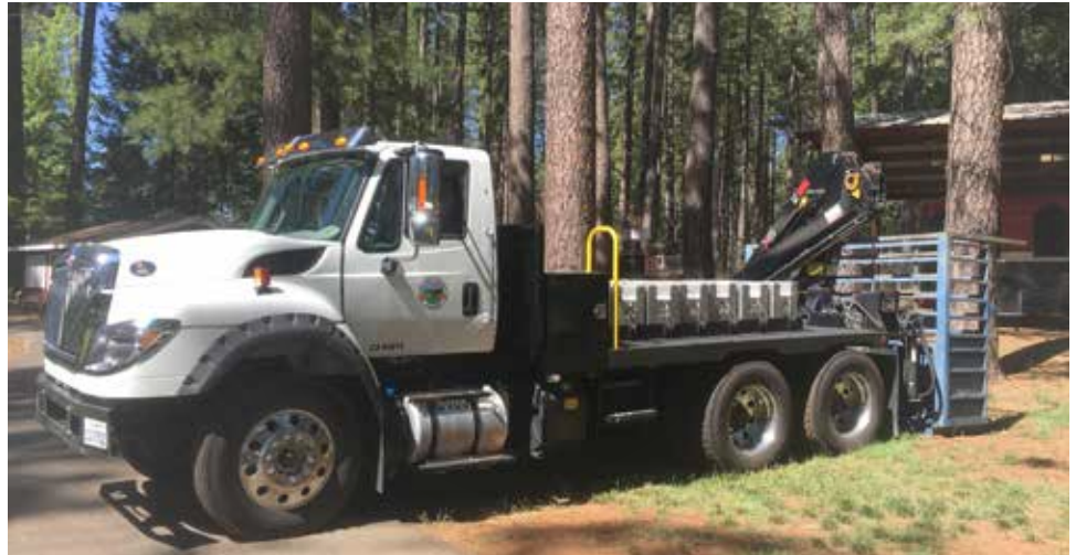
The weight truck both carries certified weights, and is a certified weight itself.
