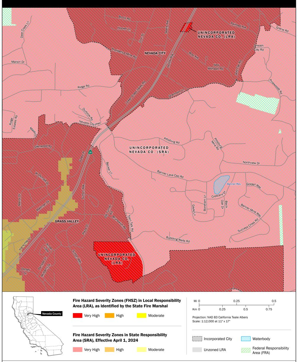
Government Code section 51178 requires the State Fire Marshal to identify areas in the state as moderate, high, and very high fire hazard severity zones based on consistent
