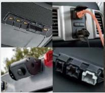
6 auxiliary upfitter switches, mounted overhead within easy reach of front-sea occurants, provide more total amos that
